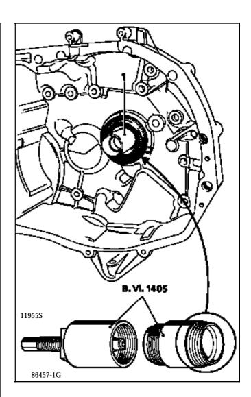
Check the condition of the smooth part of the stator shaft at (1).
