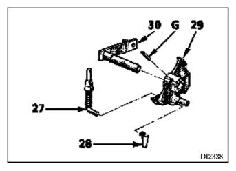
NOTE: to remove the lever (30), put it in 1st gear "hold" (opposite the "Park" position) and extract roll pin (G).
