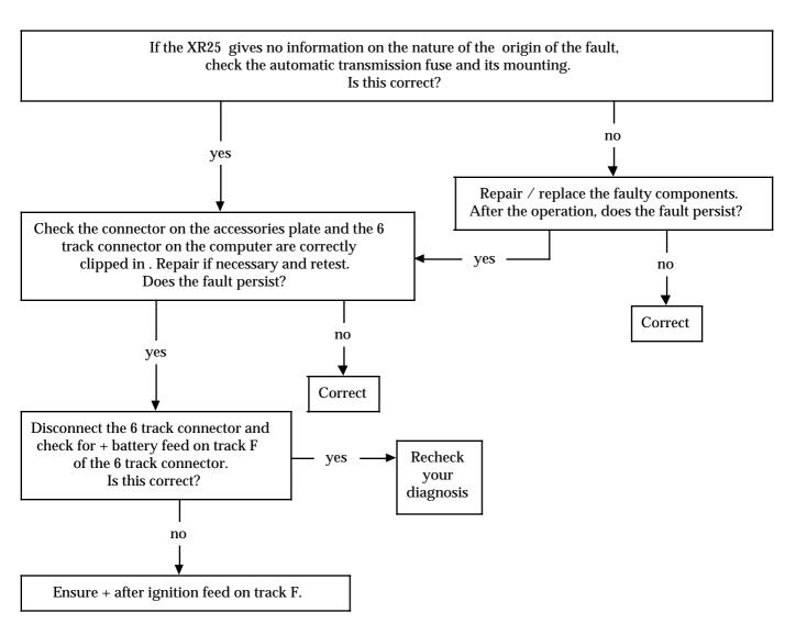
NOTE: For E7J\* engines, the fault may be caused by a break in TDC information. Check using #06 if the engine speed information changes to 0 when the fault occurs. Repair the wiring if necessary.
