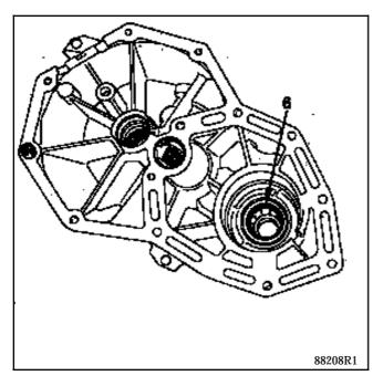
Dismantling the final drive pinion (20)
