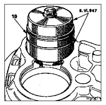
Ensure that the circlips are correctly positioned in the bearing grooves.
