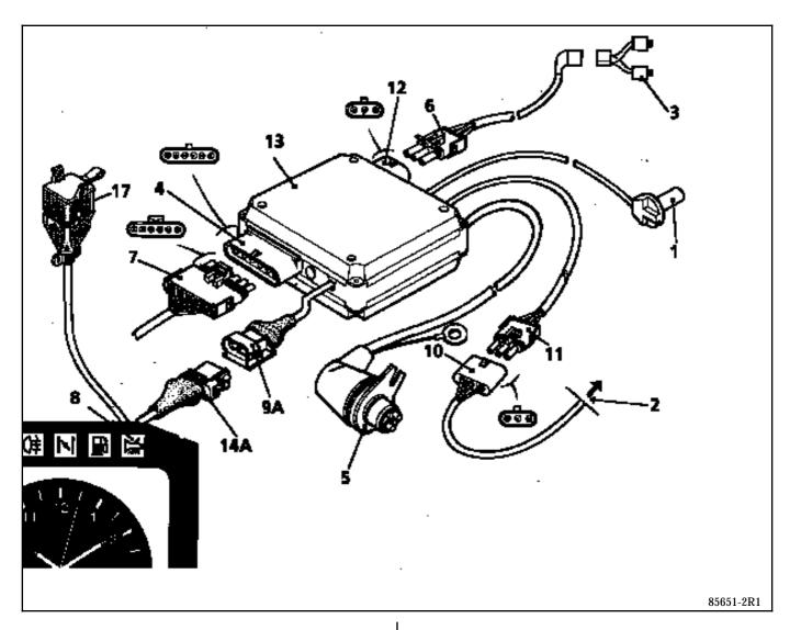
2 Connection between injection computer and automatic transmission
