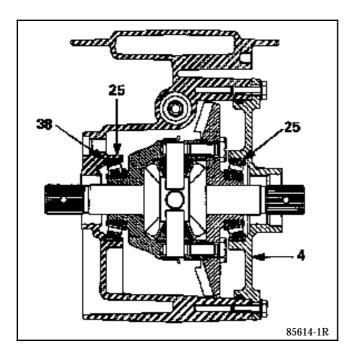
the cover plate to the differential casing and tighten to a torque of 2 daN.m.
