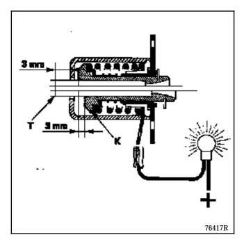
The kickdown tends to be removed and incorporated into the end of travel of the load potentiometer (no wire at D on the 6 track connector). It is adjusted by adjusting the load potentiometer (see "Fault finding" section, checking B. Vi.958).
