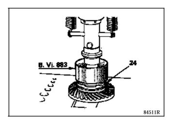
Check that the edges (A) of the band ring (24) are correctly positioned in the differential casing groove.
