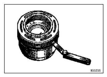
Maximum permissible clearance: MB: 3.5 mm MJ-ML: 4.1 mm
