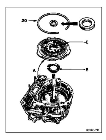
A - Offer up the assembly and rotate the reverse gear train so that the brake notches are in line with their locations.
