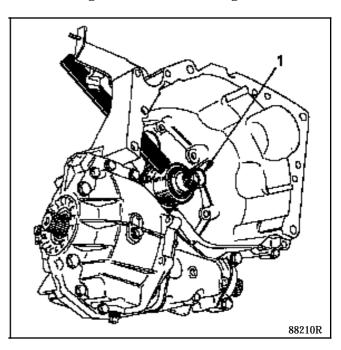
Check the condition of the smooth part of the stator shaft (1).
