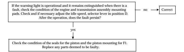
Chart 48: No 1st gear hold after operation on hydraulic distributor.
