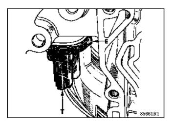
Refit the hydraulic distributor and its two seals and plate. Tighten the hydraulic distributor bolts to the correct torque in the order given (see "Hydraulic distributor" section).
