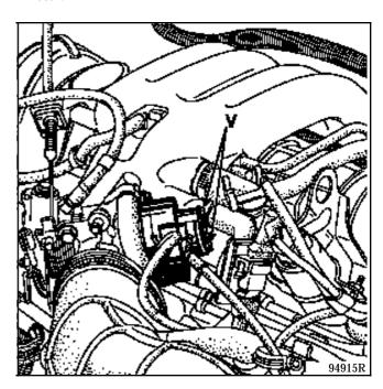
Accelerator control at rest, rotate the body of the potentiometer until a value of  $89 \pm 1$  is obtained on the display.
