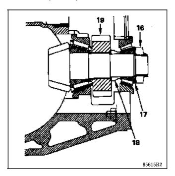
**NOTE:** For some automatic transmissions, the helical angle of the secondary pinion has been modified thus **B. Vi. 953** must be ground to modify it.
