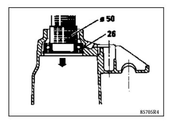
Insert a small bar inside the housing and place it flat against the bearing (R).
