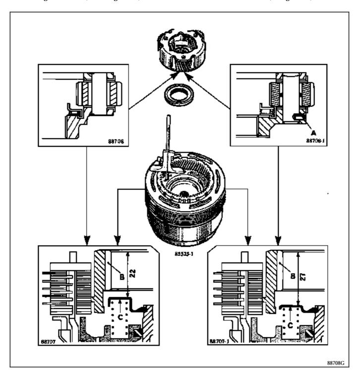
All automatic transmissions of the MB-MJ type before the **85** model may be fitted with the modified **E1-E2** assembly - identified by a dimension of **27 mm**. However, it is not possible to fit the strengthened forward gear train to an **E1-E2** assembly which has not been modified.
