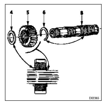
Refit part 8 and parts 4 to 6. **Ensure the pinion** (5) is the correct way round.
