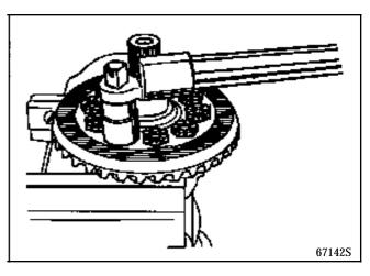
The band ring (24) is refitted on the press using tool **B.Vi. 883**, without the bearing fitted.
