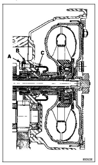
Length of pump shaft324 mmLength of turbine shaft284 mm
