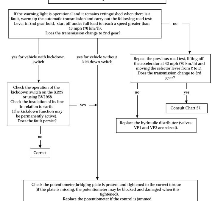
Chart 10: 3rd gear missing with racing of engine in 2nd (reverse gear correct).
