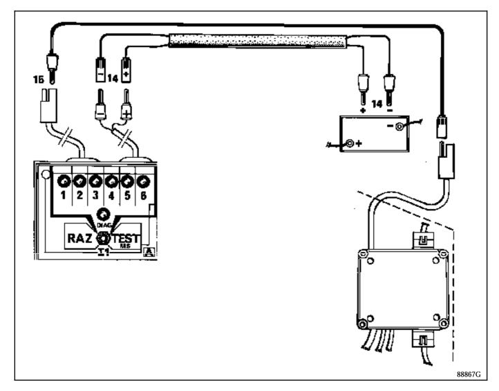
Carry out a road test and determine the faulty component depending on the illumination of lights 1 to 6.
