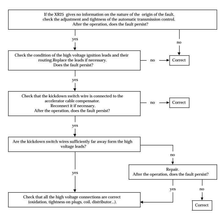
Chart 42: Gear changing thresholds delayed and warning light illuminates.
