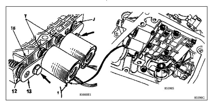
IMPORTANT: if the solenoid valves are not fitted in the correct locations, the vehicle will no longer have 1st gear.
