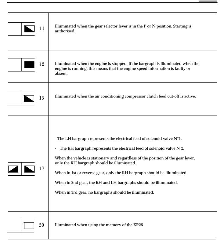
**NOTE:** To determine faults, refer to the "Fault finding charts to be used from the bargraphs" section.
