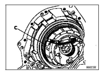
C - The operating clearance should be between 1.5 and 2.1 mm.
