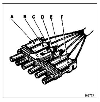
CUT THE EARTH WIRE (E) LEVEL WITH THE COMPUTER FEED 6 TRACK CONNECTOR (more than one earth must not be present).
