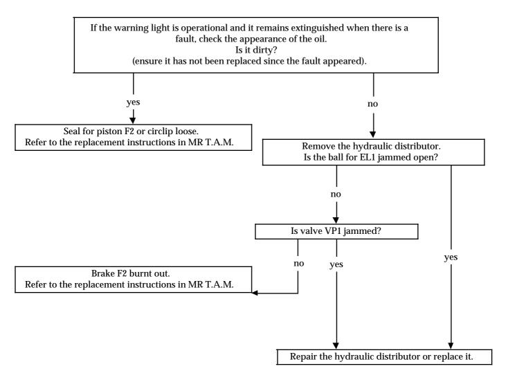
Chart 28: The engine races when changing from 2/3. the automatic transmission seems to change to neutral + no drive in reverse.
