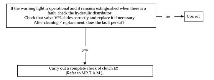
Chart 29: No reverse gear or engine braking in 1st gear hold.
