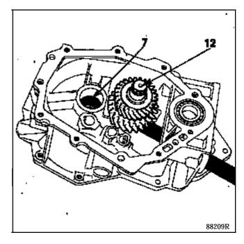
the needle bearing (7) using tool FACOM U40 and U51B or similar,
