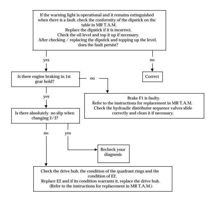
Chart 4: Skidding with engine racing when starting in position D or 2, but not in 1
