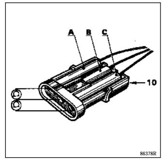
CHECKING THE THREE TRACK CONNECTOR (11) FEEDING THE POTENTIOMETER (with a voltmeter)
