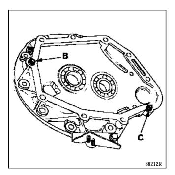
ATTENTION: all bolts mounting the separator housing must be coated with "Loctite FORMAJOINT" before being fitted.
