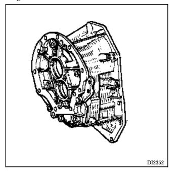
The final drive casing and the converter casing.
