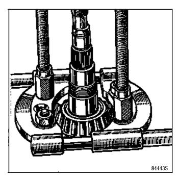
Dismantling the step-down drive shaft (12)
