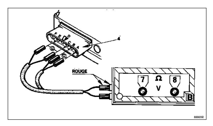
CHECKING THE LOAD POTENTIOMETER (with an ohmmeter)
