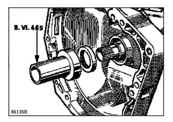
Refit the converter after having lubricated the seal face
