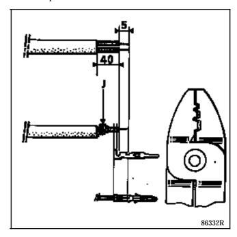
When fitting the wires in the connector, ensure that the same colours are put opposite each other.
