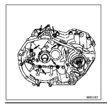
Separate the separator housing from the converter and differential casing.
