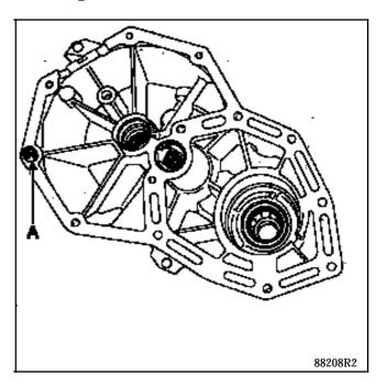
**IMPORTANT:** the two bolts under the stator shaft must be coated with "**Loctite FORMAJOINT** ".
