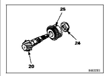
Fit the bearing (25) using the press with the mark at the final drive pinion end.
