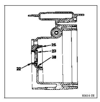
With a small lever, release the outer track ring (25) and use tool **Mot. 587** to finish the operation.
