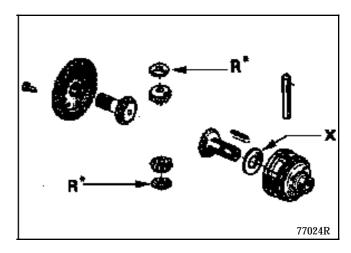
Attach the washers (R) to their respective planet wheels and recover the adjusting shim (X).
