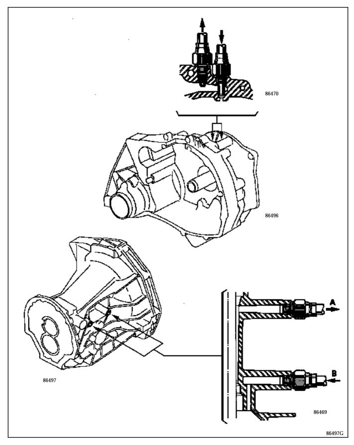
Blow compressed air into the oil cooler inlet and return pipes (A and B).
