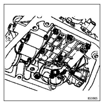
Fit the sump and tighten the bolts to a torque of **0.6 daN.m** (except on **ML**).
