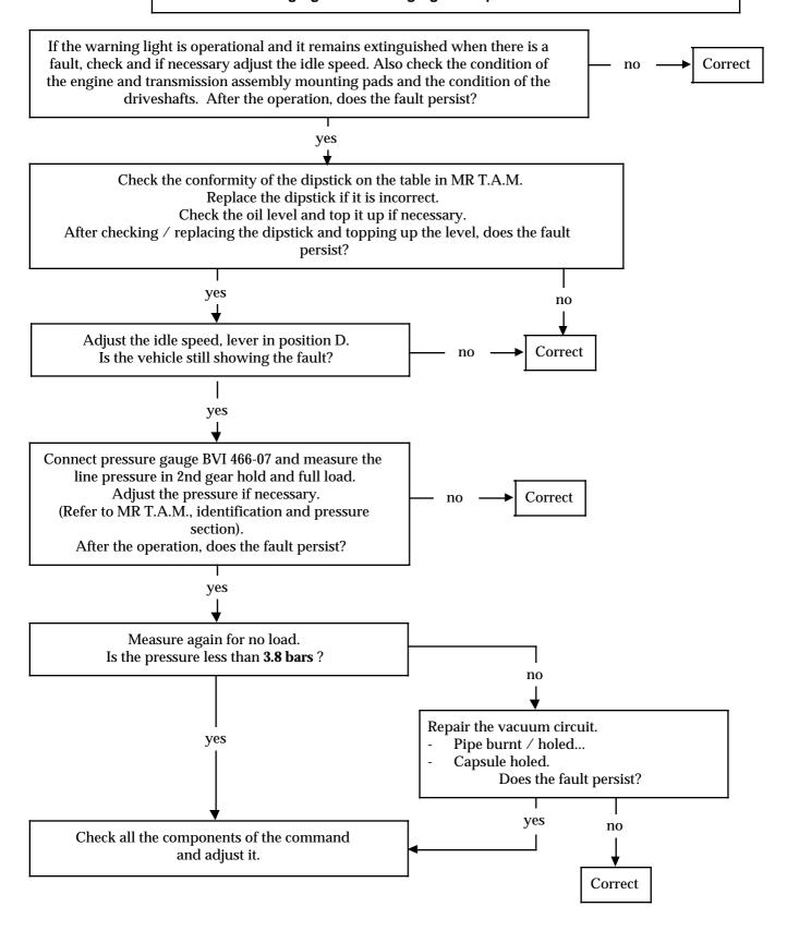
Chart 17: The vehicle moves forwards or backwards with the lever in N and the starter motor and reversing lights positions are offset.
