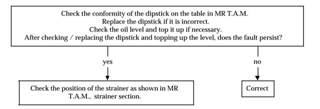
Chart 39: Vibration at 37 - 50 mph (60 - 80 km/h) or humming on flat road.
