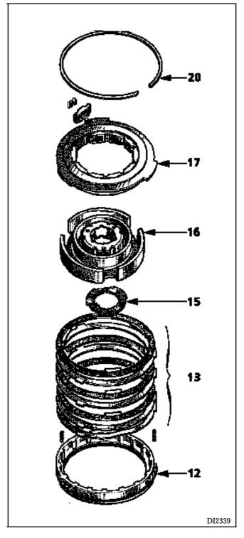
the piston (12) blowing compressed air through hole T (see next page),
