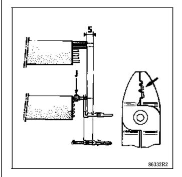
When refitting the wires in the connector **ensure** the same colours wires are connected opposite each other.
