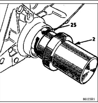
Seal (28) is refitted using tool **B. Vi. 945** which consists of:
