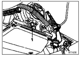
Connect pressure gauge **B. Vi. 1215-01** (before using the device, **reset the pressure gauge to zero**).
