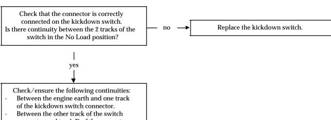
Between the other track of the switch connector and track D of the computer.
