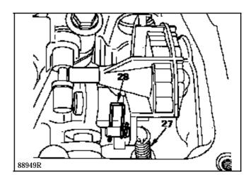
Fit clip (E) to the sealed connector (T) and connect it
