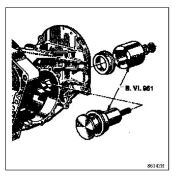
Refit the inner bearing track ring to the final drive pinion (20).
