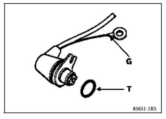
Check the presence of the O-ring (T) and fit the multifunction switch on the automatic transmission.
