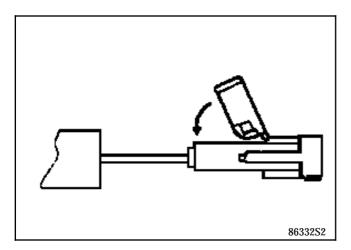
There are computers connected to multifunction switches by seven wires and, in this case, cut the 7th wire (yellow or white) level with the sleeve on the computer side.
