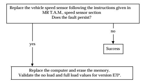
\* And vehicles with load information supplied by the injection computer. (Without load potentiometer specific to the automatic transmission).
