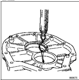
The differential should rotate under a load of between 3 and 6 daN.m, in the case of new bearings and freely, without play, when the original bearings are refitted.
