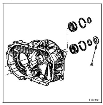
Leave spacer (E) and shim (K) on the output shaft.
