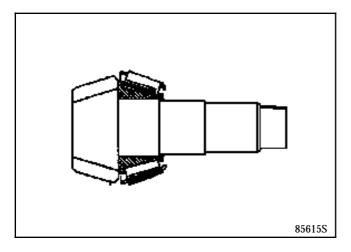
Offer up the final drive pinion (2) to its location on the final drive casing and fit:
