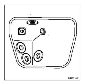
\* Direction for fitting magnets: ribbed side against plate
