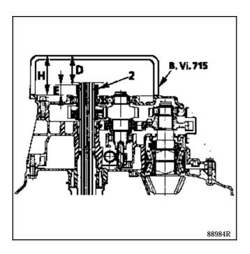
3 - Calculating the thickness of the shim (K).
