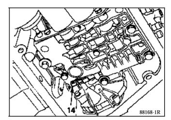
Refit the sump equipped with a perfect gasket.
