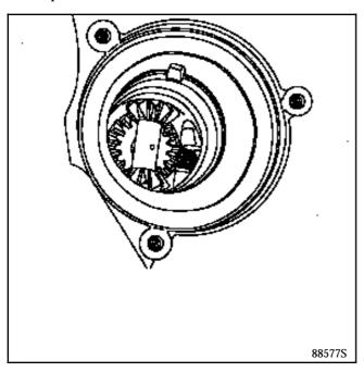
Loosen the pinion with a screwdriver and recover it.
