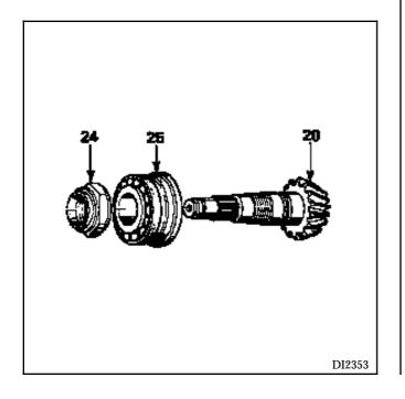
Using an extractor, extract the bearing
