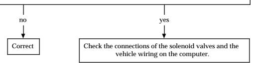
Chart 47: No reverse gear when warm or bang when engaging reverse when reaccelerating.
