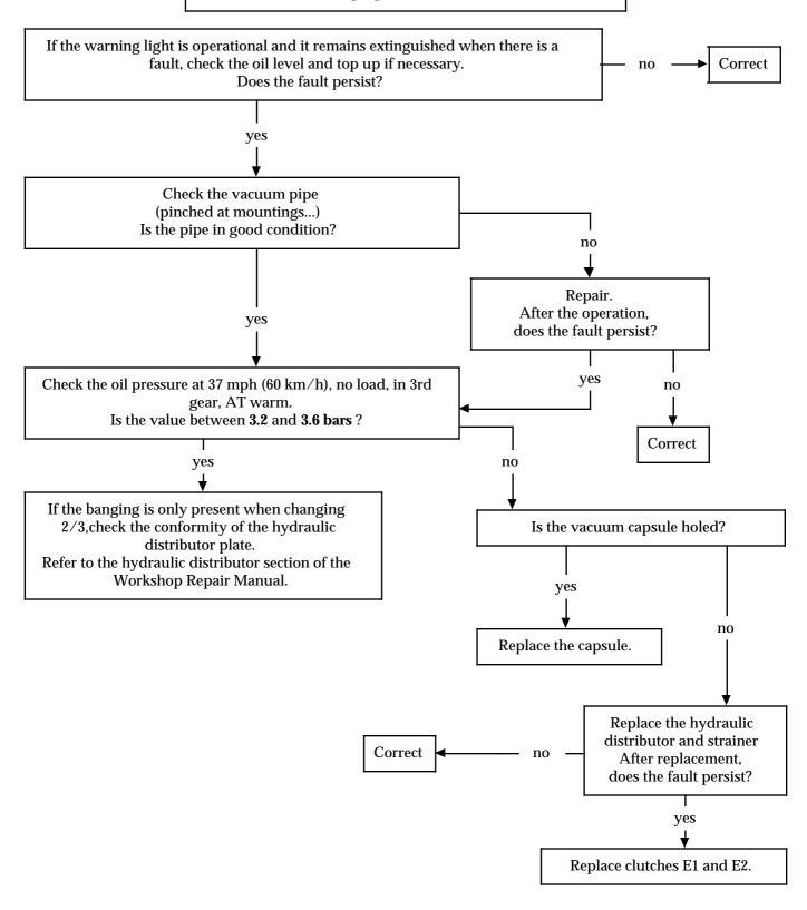
Chart 14: Slipping when changing gears in full load position
