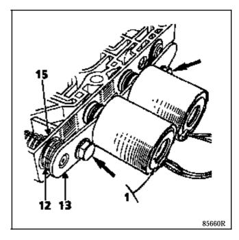
Tighten the bolts securing the cover plate (13) progressively so that the last coil of the spring (12) is not jammed between the plate (13) and the unit (15) and tighten to a torque of **1.3 daN.m**.
