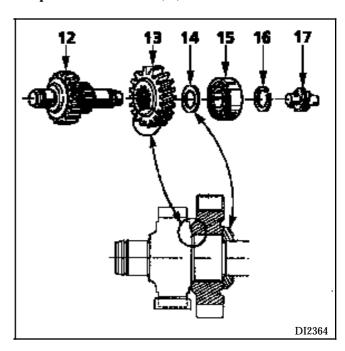
Refit parts 12 to 17 (15 and 13 using the press). **Ensure pinion** (13) **is fitted the correct way round**.
