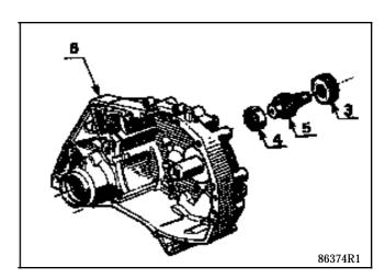
Extract the bearing using an extractor (example FACOM U49).
