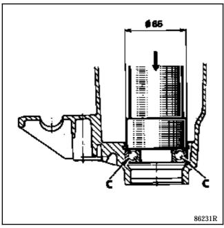
Replace the circlip which holds the bearing.
