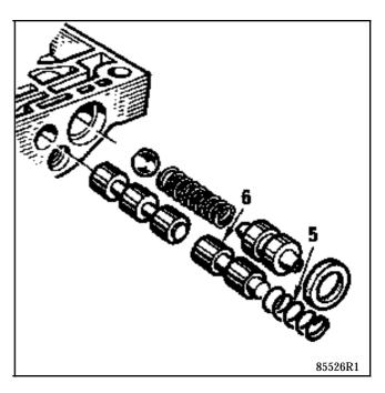
Secure plate (13) by its two bolts and fit the solenoid pilot valve with mark (1) at the same end as the pressure regulating valve.
