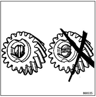
Fitting the differential in the casing.
